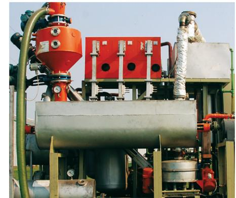
Biofuels can be produced from oilseeds such as sunflower, flax, and safflower (top). A mobile, pilot-scale microwave-assisted pyrolysis system like the one shown here lets the University of Minnesota perform biofuels research outside of the laboratory (bottom).
